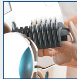
VITEK® 2 COMPACT: Cards inoculated inside instrument and manually transferred from filling door to loading door for processing
